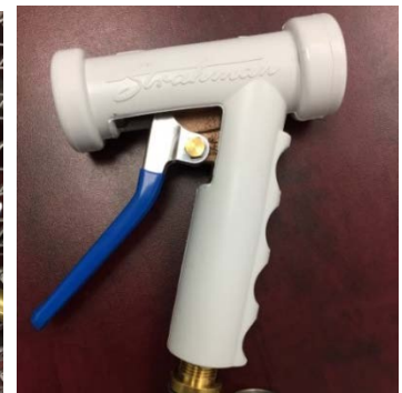
After – New spray gun(red, 29.3 LPM at 80 psi), Newest spray gun (white, 18.5 LPM at 80 psi)
